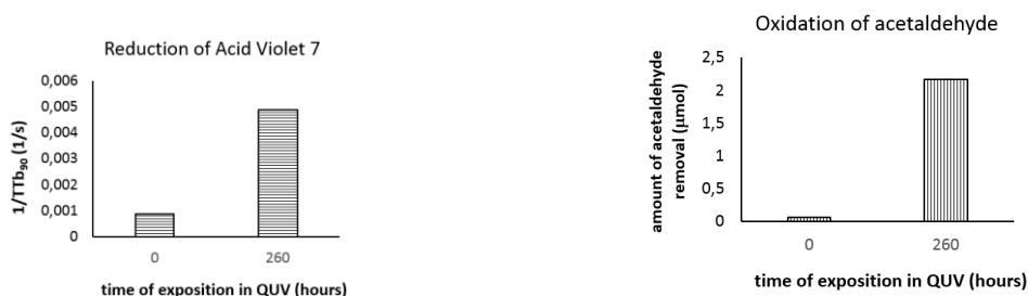
Figure 1.: Rate of photocatalytic reduction of AV7 (on the left) and rate of photocatalytic oxidation of acetaldehyde (on the right)
